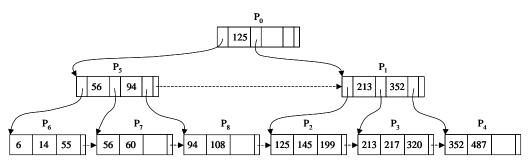
Figure 6.18 The B-Tree of Figure 6.17 After Inserting 60 Page  $P_7$  is split into  $P_7$  and a new page  $P_8$ , links are updated, and the boundary key 94 is inserted in page  $P_5$ .
