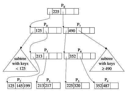
**Figure 6.6 A B-Tree After a Recursive Split** This shows the B-tree of Figure 6.15, after inserting key 225, assuming  $P_1$  can hold at most 2 keys. Thus,  $P_1$  must split into  $P_1$  and  $P_6$ , which in turn causes  $P_0$  to split into  $P_0$  and  $P_7$ , which causes a new root  $P_8$  to be created.
