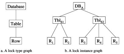
**Figure 6.19 Graph that drives multigranularity locking** The lock type graph describes the hierarchy of granularity of object types that can be locked. The lock instance graph shows instances of those types.
