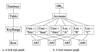
**Figure 6.21 A DAG that Drives Multigranularity Locking** This extends the graphs of Figure 6.19, to allow each row to have more than one parent, which in this case are key ranges.
