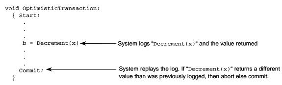
Figure 6.5 Using a Decrement Operation with Optimistic Locking No locks are set when Decrement(x) first executes. During the replay of Decrement(x), the system sets locks, but aborts if the result changed since the original execution.
